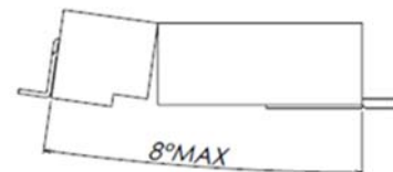
图 2/ Fig.2(水平对接型/Horizontal connection type)
